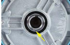
Identify the stroke of the crankshaft.
