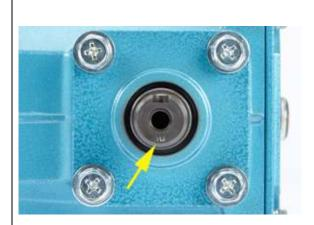
Identify the stroke of the crankshaft. This is printed at the location shown above
