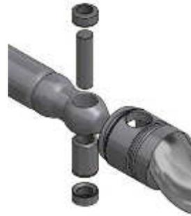
**Maintenance:** The RL Series is designed to ensure easy maintenance, with only a minimum number of replacement parts necessary. In particular the bushings on the joint enable it to be completely replaced without having to replace the shafts and rotors. Maintenance costs are thus reduced. The cost of the machine is also highly competitive, considering its entire life-cycle.
