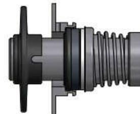
**Modular Design:** The RL Series is based on a modular concept in every single feature: hydraulic parts, casings, seals, stands, supports and drive shafts. Each component can be constructed in a number of variants without modifying the structure of the machine, thus maintaining standard key replacement components.
