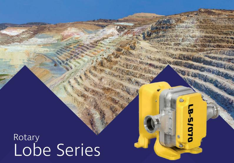
Boyser Lobe Pumps are available with either Rubber or Metallic lobes ensuring suitability for a range of Fluids. Producing a maximum pressure of 10 bar and flows up to 92M³H, they are designed for industrial and hygienic applications which require a low shear pumping motion, high flows, with a continuous non pulsating flow in a compactly designed unit. Liquid temperatures of up to 120°C can be accommodated.
